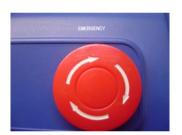
**DEAD MAN SWITCH PUSH** for OFF – for normal operation **PULL for ON**
