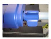
PADDLE LEVER Push lever forward for forward motion. Push lever down for reverse motion. (Buzzer should sound in reverse) FORWARD MOTION IS ALWAYS RECOMMENDED!
