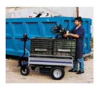
ZALLYS HT - Our 3 wheel electric pedestrian operated tiller head unit is equipped with a sturdy tubular steel frame and powder coated with exterior paint, able to be accessorized with various type of containers, or platforms, easy to be installed and interchanged. Ecological and silent, guarantees speed in all types of stocking and warehousing works.
