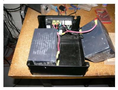
2. Place Battery B into the box making sure the wires are nested between the batteries and that no wires are detached. The fit is designed to be tight.
