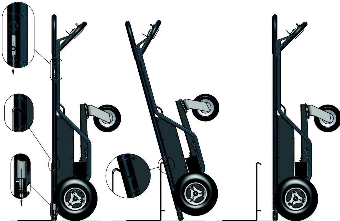
Tool attached and locked
