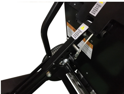
Stowed Position Detent pin in stowed hole
