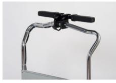
Grip the handle to activate the power assist. The assist function works only when you are holding the handles, if you take your hands off, the brakes will automatically apply.
