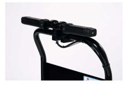
Grip the handle to activate the power assist. The assist function works only when you are holding the handles, if you take your hands off, the brakes will automatically apply.
